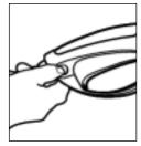
Step 6 Disconnect the high pressure hose from the high pressure outlet and engage the gun safety lock.
